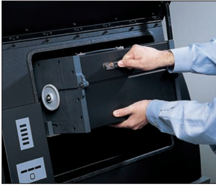
With daylight-loading material cassettes, no time is required in the darkroom.
