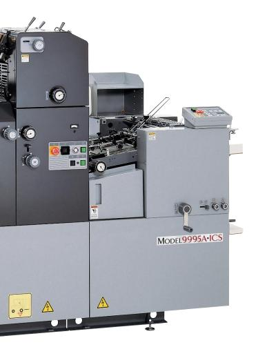
Model Shown: ABDick 9995A-ICS with Semi-Automatic Plate Inserter and Inking Control System
